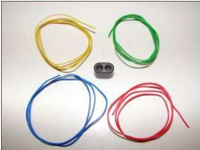
First prepare some 25cm / 0.5mm core diameter kynar/teflon wires.
